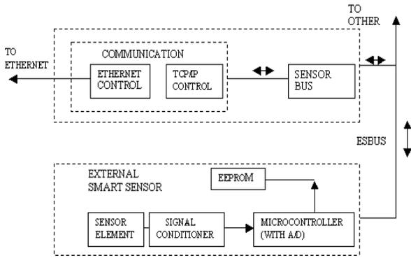
Fig. 1 Block Diagram of a Networked Sensor
