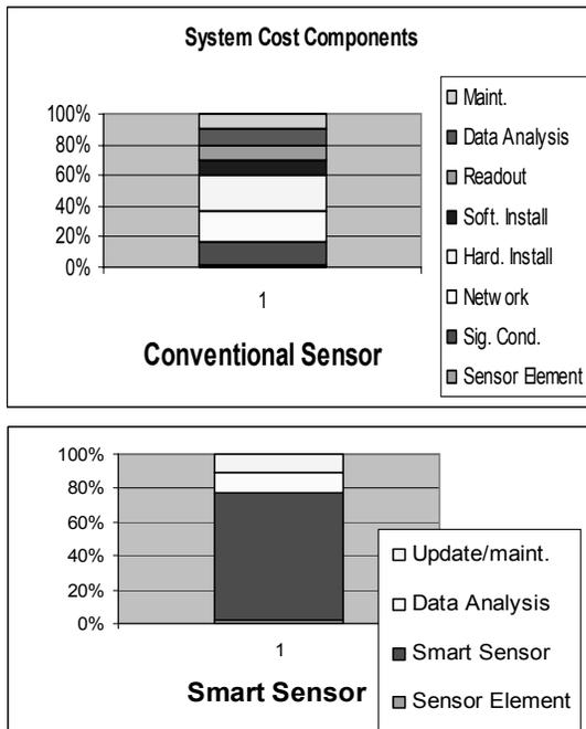
Figure 7 Smart Sensor Cost Comparison
