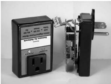
Fig. 2 Integrated ES02 module with the plug-in case
