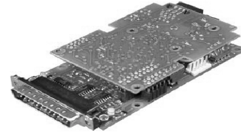
Fig. 3 EM02 module. Communication (TCP/IP & Ethernet) is on top
