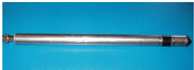
Figure 8. Photo of Soil Moisture Sensor in Case
