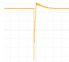
Fig. 6. Measured Transmitter Transducer Waveform
