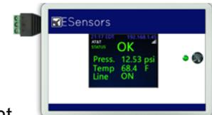
The gateway accommodates any of these common sensor signals: 4-20 mA current, 0-5 volts, pulse (0 to 2kHz) or switch (pull-up/down or dry contact). A hardware multiplex circuit (MUX) section, normally factory-configured, adapts the module to the proper analog signal. The sensor type (e.g. pressure), units (e.g. PSI) and full scale (e.g. 15) are set by a configuration page. Actuators (relay, LED, LCD display) are also accommodated.
