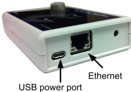
Figure 3 – Location of Wall Supply connector.
