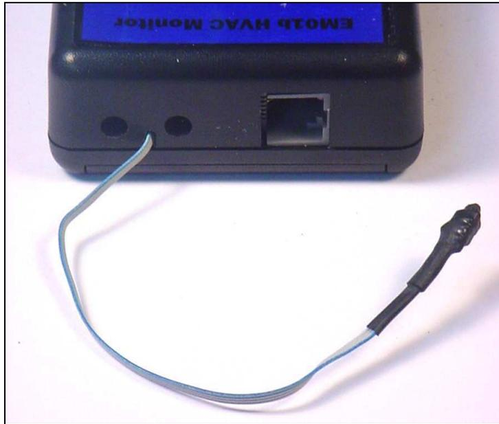
Figure 24 - Websensor's tail (temp/RH sensor).
