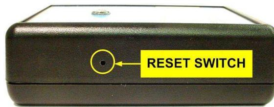
Figure 8 – Location of RESET PUSHBUTTON.
