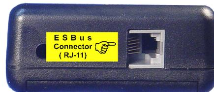
Figure 6 - Eibus Connector (RJ-11).
