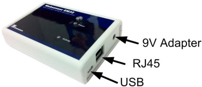
Figure 5a – Location of RJ45 and Wall Supply connectors.
