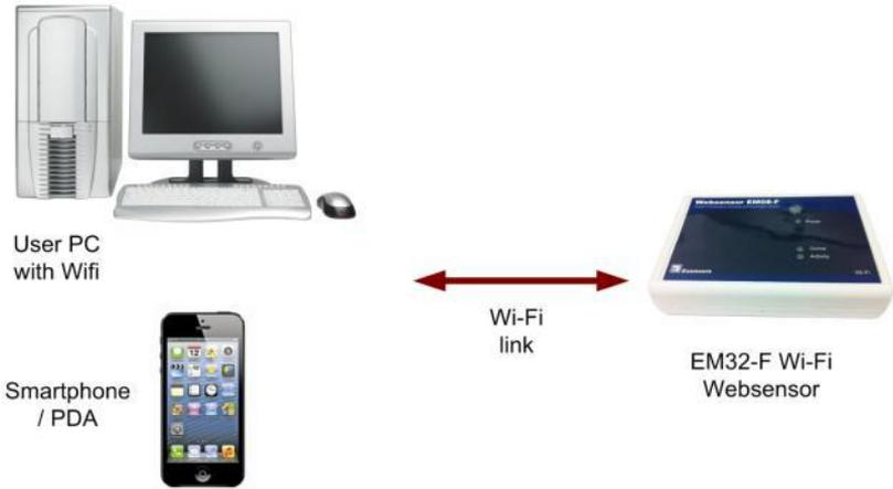
Figure 5. EM32-F connected straight to a PC/ cell phone.
