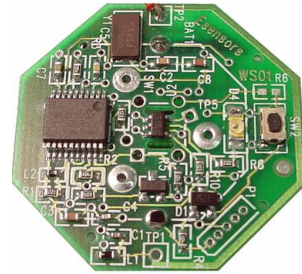
Fig 1. Transmit-only Wireless Sensor Circuit Board
