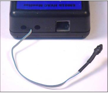
Figure 24 - Websensor's tail (temp/RH sensor).
