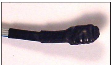
Figure 25 - Close-UP of the temperature/RH sensor.
