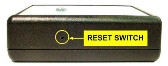
Figure 21 – Location of the RESET button on the Websensor.
