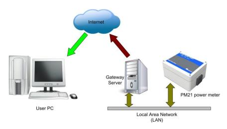
Figure 2 – How the PM21 works.
