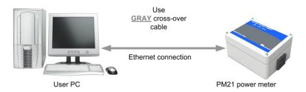
Figure 4 – PM21 connected directly to the NIC in a PC
