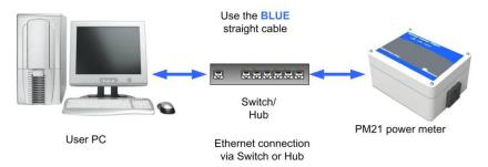
Figure 5 – PM21 connected through a HUB to the NIC in a PC.
