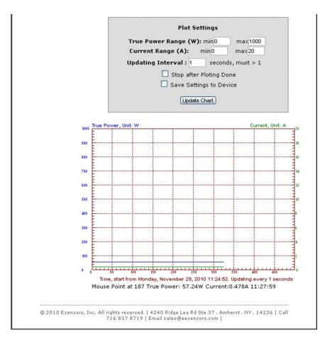
Figure 9 – Visualizing Outputs screen (Data collected with an incandescent bulb rated at 120V 60W as load)
